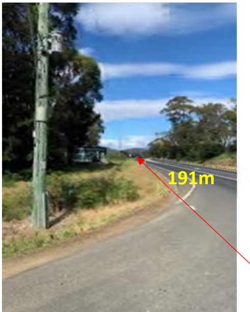
Figure 28: Sight Distance at the Tasman Highway/Pittwater Road intersection was measured to be approximately 191 metres to the left (West).
