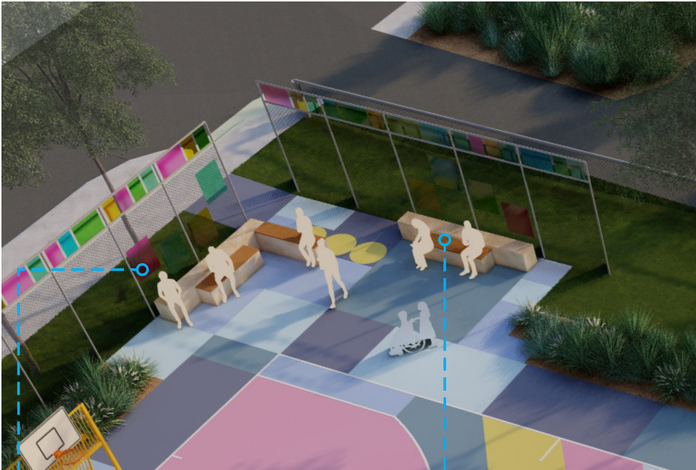
Feature Fence Steel post & wire fence with colourful plexiglass sheets for transparent wind protection. Posts can be powdercoated for pops of colour. Posts behind goal posts could have chainwire mesh for ball rebound net
